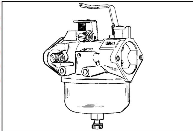
Choke lever positioning is maintained by the stop spring, replace if damaged.
