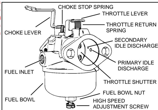
Install the throttle plate with the numbers (if present) facing out when closed. Move the throttle shaft to the closed position, place the throttle plate on the shaft and secure with the retaining screws. The throttle should move freely. If binding is present, correct by loosening screws and repositioning throttle plate.
