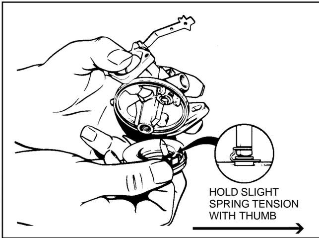
Position the choke shaft and shutter in the closed position prior to tightening the screws. Hard starting may be due to insufficient choking action because of a misaligned choke plate. Correct by readjusting choke plate to close completely.
