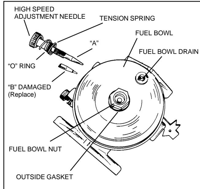
Use new gaskets when rebuilding the carburetor. If the fuel bowl to carburetor body gasket does not seat, enlarge by stretching with 4 or 5 quick short strokes. Fiber gasket must be used between center of fuel bowl and carburetor body.
