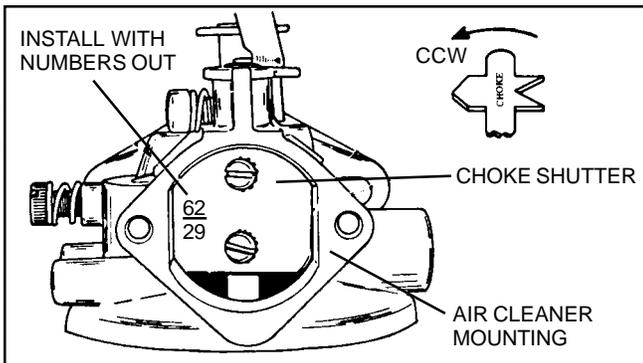
Figure below shows a typical choke shutter found on vertical engines. The full choke position of the choke lever is clockwise when viewing from the top of the carburetor. Note cut-out position of choke shutter.
