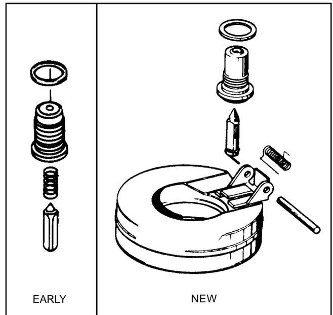
This shows early and new needle valve, seat, gasket, and spring assembly for large horsepower engine carburetors.
