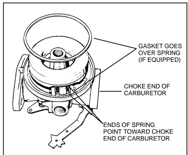
When assembling the float to the carburetor body, position the needle spring on the adjusting tag so that it hangs down. Hold the float spring under tension until the carburetor body will support the slight spring tension.
